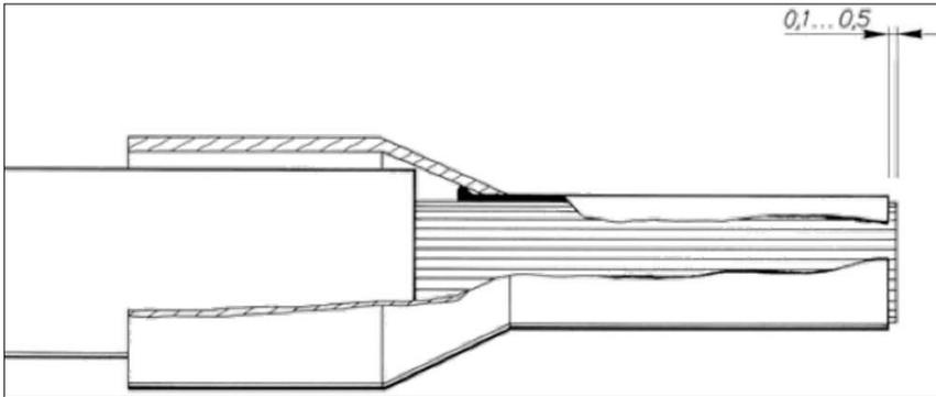
As shown in the illustration, the conductor insulation must be pushed into the plastic collar, and the conductor should completely fill the ferrule sleeve. Depending on cross-section, the conductor should protrude as much as 0.5 mm from the ferrule sleeve.
