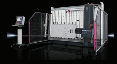
While you are at the Oil and Gas Competency Center, you can discover the Perforex machining unit which was designed to automatically create holes, threads, and milled surfaces on all standard materials including steel, stainless steel, aluminum and copper.
