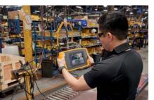
The ii900 Sonic Industrial Imager lets technicians see sound as they scan hoses, fittings and connections for leaks. Its built-in acoustic array of tiny sensitive microphones generates a spectrum of decibel levels per frequency. Based on this output, an algorithm calculates a sound image, known as a SoundMap, which is superimposed on a visual image. The SoundMap is automatically adapted, depending on the frequency level selected, so that background noise is filtered out.
